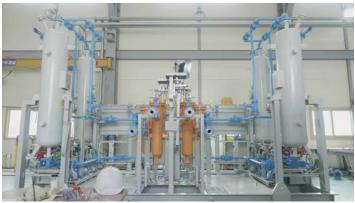
These compressor and dryer packages were built according to API specifications
