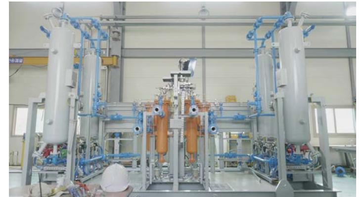
These compressor and dryer packages were built according to API specifications
