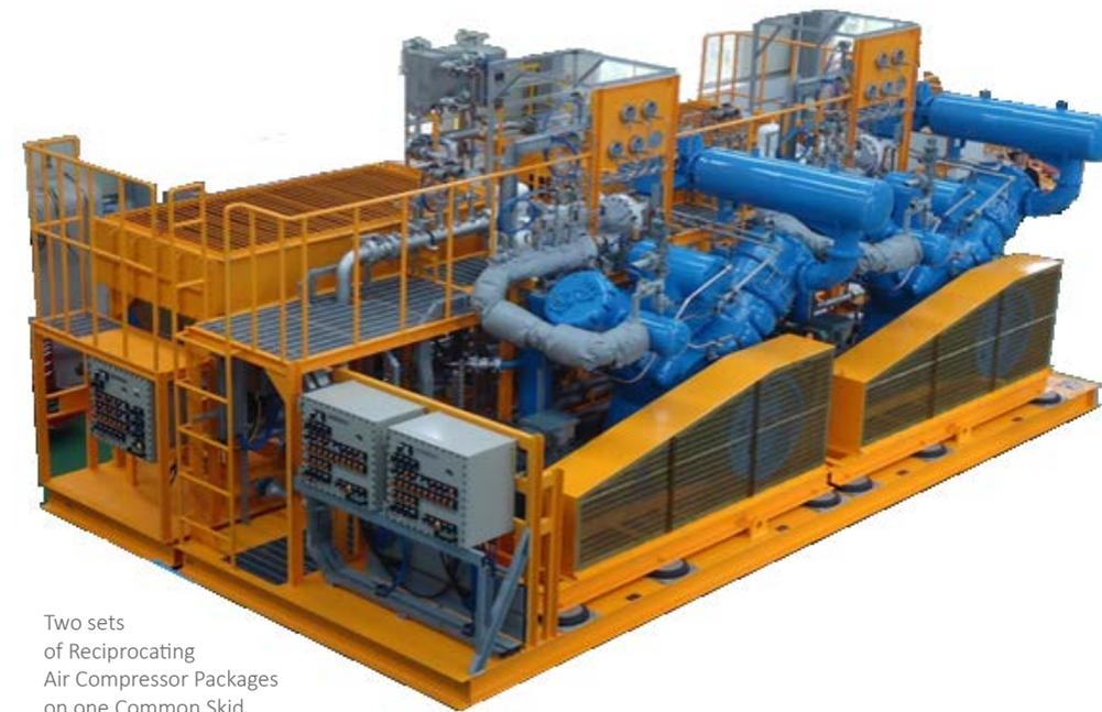
Two sets of Reciprocating Air Compressor Packages on one Common Skid
